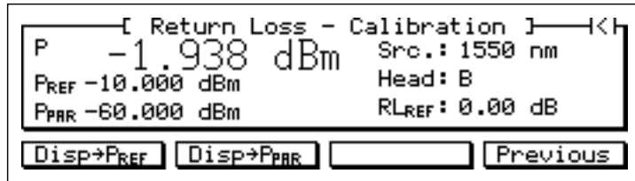
Figure 3-5 Return Loss Calibration Display
